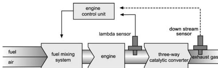
To further improve control of exhaust emissions most vehicles produced after 2000 have an additional Lambda sensor fitted down-stream of the catalyst that monitors the performance of the catalyst itself.
